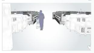
Single side operation streamlines and optimizes the traffic flow of operators. This increases efficiency in supplying materials and performing maintenance
