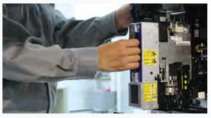
Fuii's original compact lightweight heads that can be easily exchanged without using tools. Operators on-site can perform maintenance and handle troubles.
