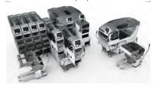
Modules, heads, and supply units can be freely exchanged based on changes in the part types and production types. This is a unique mechanism that maximizes production in the given floor space.
