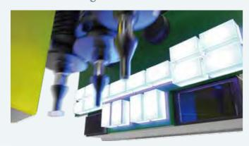
Checks tombstoned parts, missing parts, and up-side down parts
